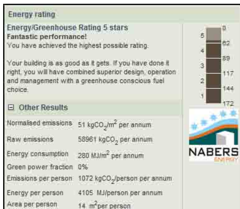
Figure 2: NABERS Rating Output - produced from NABERS Office Rating Calculator
